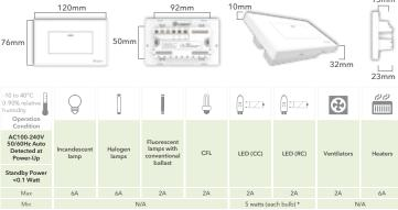
\* For 2-wire (without neutral wire) installation only. Please wire the LED power you encountered conditions of circuit instability, lightings gleaming or no light
