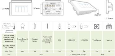
\* For 2-wire (without neutral wire) installation only. Please wire the LED power stabilizer if it is required to work with LED bulbs in 5 watts below when you encountered conditions of circuit instability, lightings gleaming or no light.
