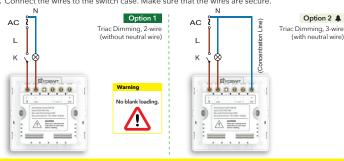
By default, the dimmer setup of the switch is in 2-wire Triac Dimming. If you attemp to use other wiring method, e.g. 3-Wire Triac, 0-10v, 1-10v, please complete the setup in the app (1. Assign the device to room, 2. Choose the suitable wiring in device setup page) after wiring.
